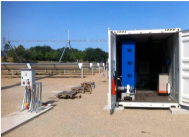
MHD technology, developed by TMW, can treat any kind of polluted waters: high salinity waters, brackish waters, acidic or basic waters... It can extract pure water available for human consumption. This process maximizes pure water production if we compare it with alternative desalination processes such as reverse osmosis. MHD doesn't need any heavy infrastructure and can be operated as a stand-alone, autonomous unit using any kind of energy (solar PV or thermal...), and no fuel consumption.
