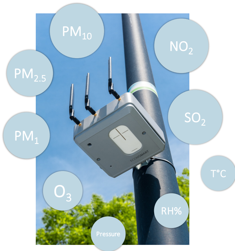
ECOMSMART Ambient air connected measuring station
