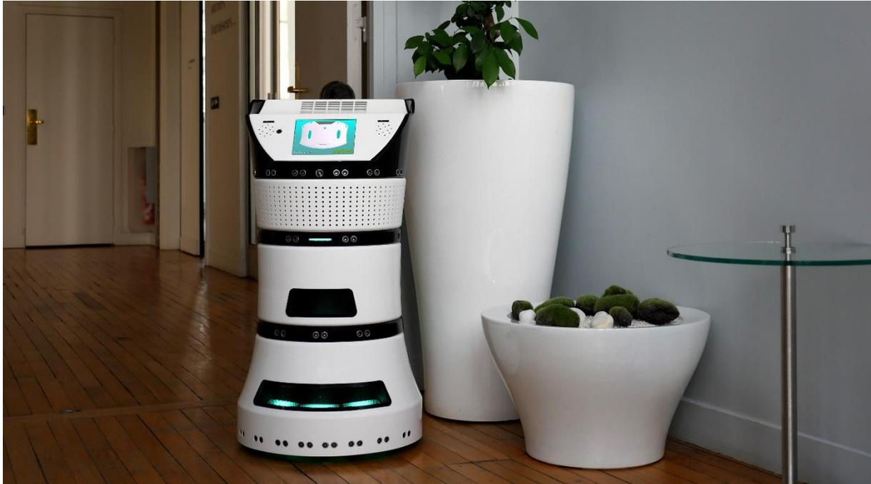
Diya One X is a non-humanoid robot with an artificial intelligence based on a neuro-inspired model. Thanks to this unique AI he is able to autonomously navigate in large and highly dynamic environment (5 000 to 11 000 sqf) without lasers or a prerecorded map, a first worldwide.
